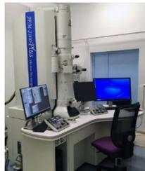
**New 2018 : Cryo- transmission electron microscope**
